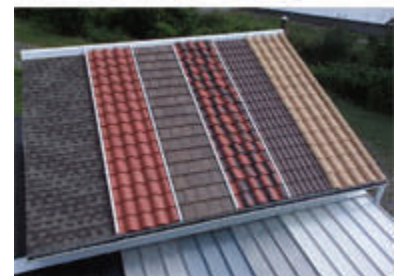
Types of Cool Roofing Materials
